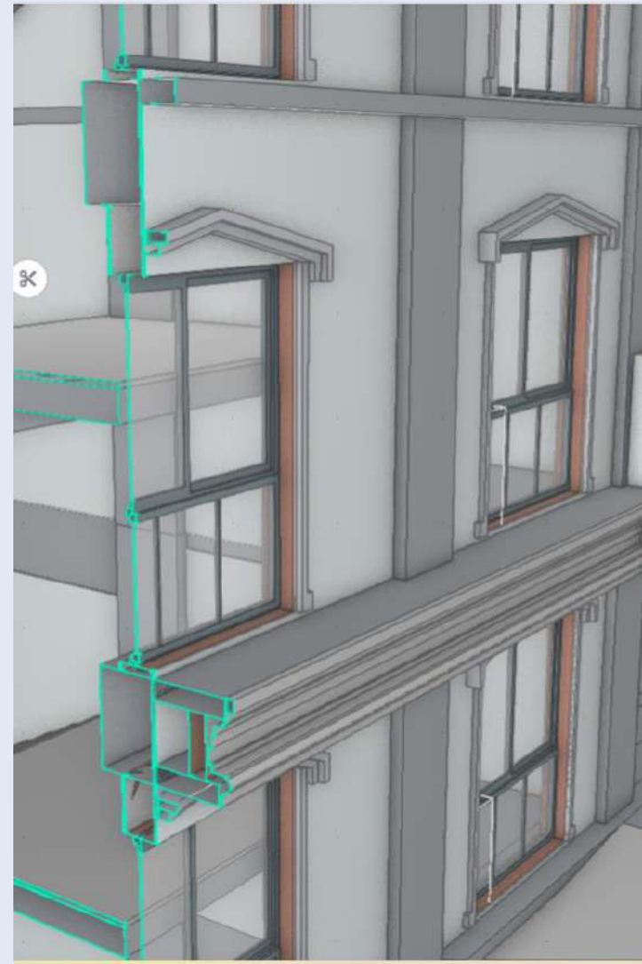
Coordinated Architectural and Structural Design Processes
